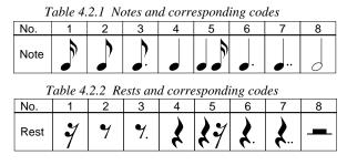
Eight notes can be specified with the 3 bits melody data. Fill in the note field with numbers from 1 to 8.
